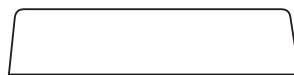
Figure 13: Fiber paper thickness too great Dams not vertical—finished block won't sit vertically.
