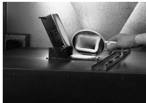
FIGURE 7: USING A MIRROR TO CHECK FOR CONDENSATION.
