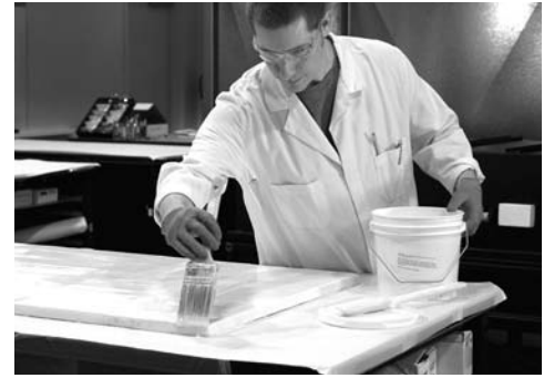
FIGURE 8: BRUSHING QF-180 ONTO THE FIBERBOARD SHELF.
