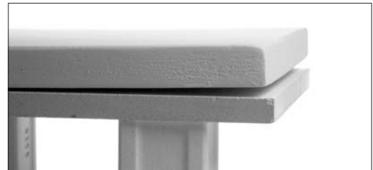
FIGURE 12: EXAMPLE OF A BOWED FIBERBOARD SHELF CORNER.
