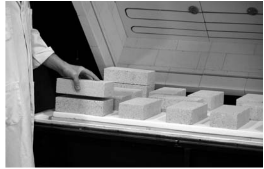
FIGURE 11: WEIGHTING THE FIBERBOARD SHELF WITH BRICKS.
